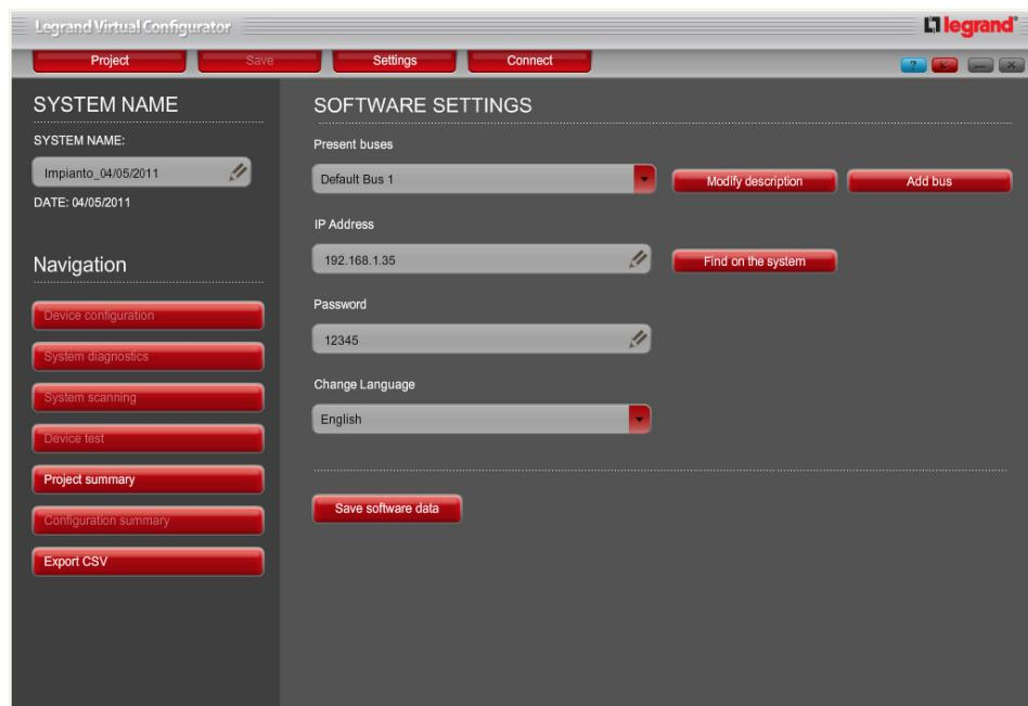
When the program is started, the screen shows the Settings menu as active. At this stage network connection has not yet been established (the "connection status" icon is red), and only "Project Summary" and the "Export CSV" are enabled.
