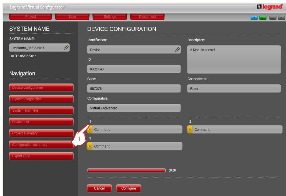
On the top of the screen is a summary of the device being configured, with a Description, the device ID, the Item code No., the connection, and the configurators.
