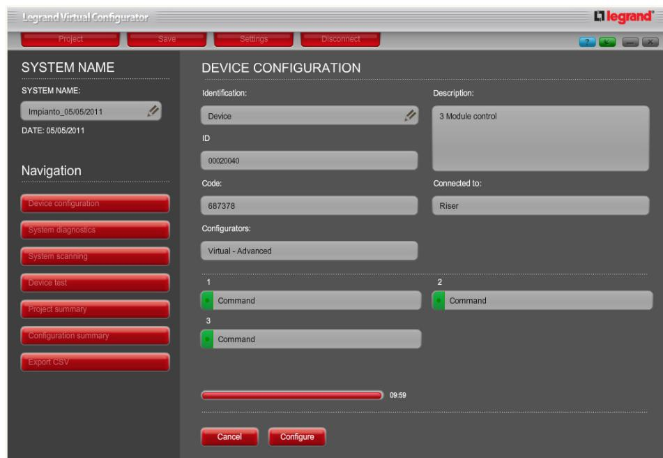
Once all the configuration operations have been completed, press **Configure** to send the configuration to the device.
